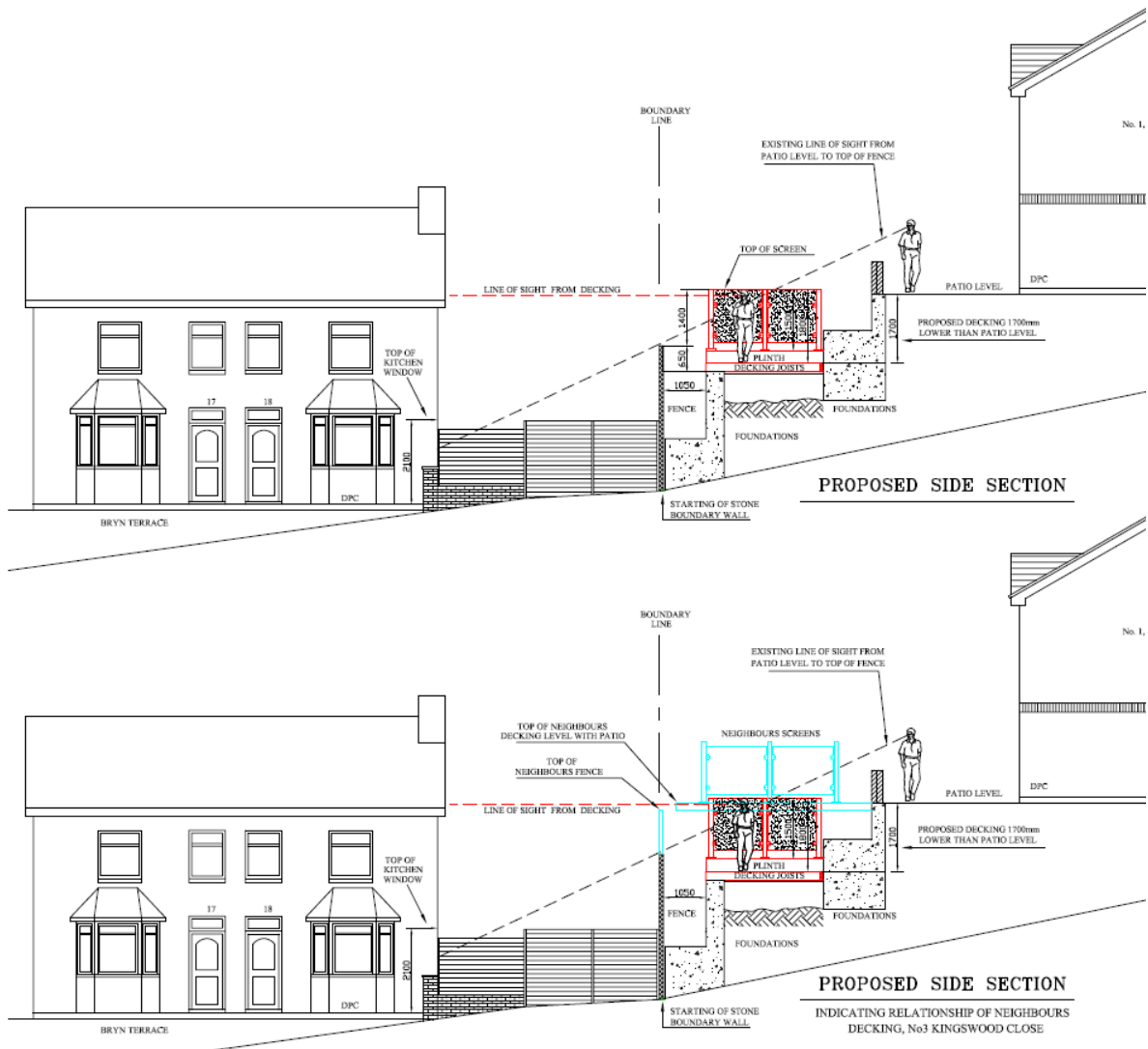
Figure 1. Revised side section indicating a 1.8 metre privacy screen and relationship of neighbouring sun deck to no. 18 Bryn Terrace
